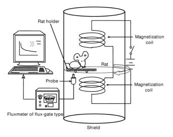
Figure I Lung magnetometric evaluation apparatus.
